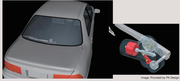
Worm gear used for the oscillating mechanism of wipers
