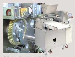
KWGDL Duplex Worm Wheels and AGDL Worm Wheels used for indexing and driving, for accurate filling of a fixed amount of ingredients
