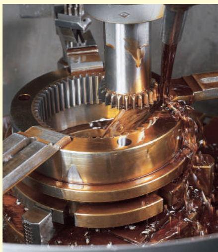
Gear cutting by CNC Gear Shaper
