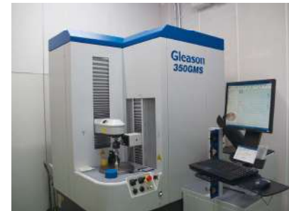
Gear Measuring System (350GMS)
