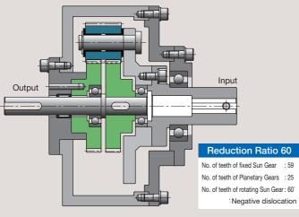
Mechanical Paradox Gear Mechanism used in a large reduction gear
