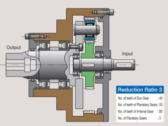
Planetary Gear Mechanism used in a reduction gear
