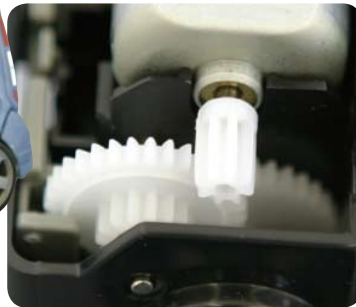
Gears transmitting power and motion to the tires.
