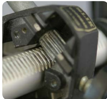
A round rack and a pinion
