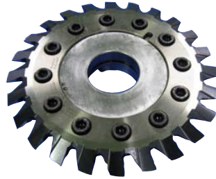
Coniflex cutter (the lower cutter)
