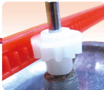
A belt-shaped rack and a gear to spin the top
