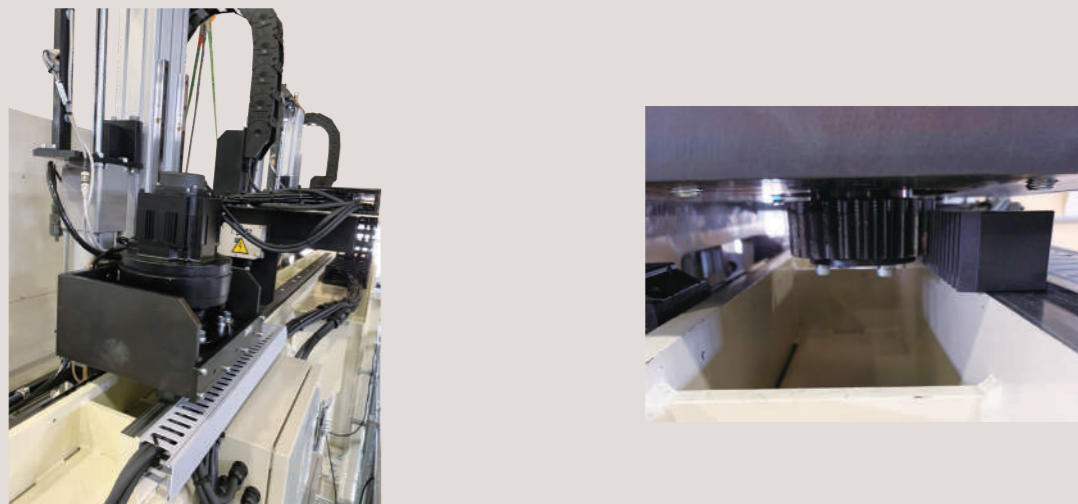
SRCPF-H racks and SSCP spur gears used in cleaning device with automatic transport for automobile parts
