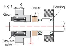
Clearance (Assembly conditions require clearance of 1 mm or more)
