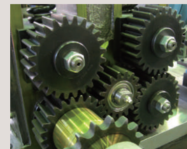
SS spur gears used for wire feeder
