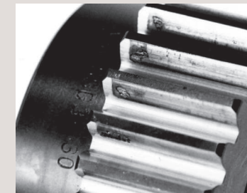
Poor tooth contact and pitting
