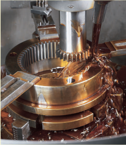
Gear cutting by CNC Gear Shaper
