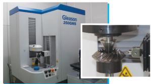
Gear Measuring System (350GMS)
