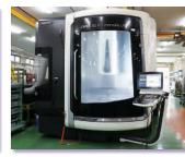
Combined Machining Machine (DMU 85 FD monoBLOCK)
