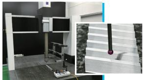
Carl Zeiss 3D Coordinate Measuring Machine (ACCURA)
