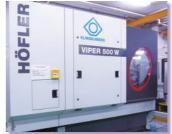
Gear Grinding Machine (VIPER500W)
