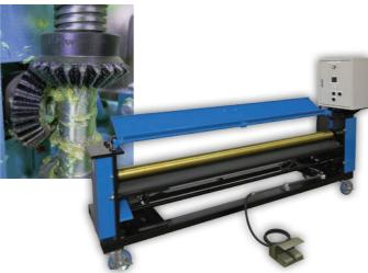
Uses SMA miter gears for bending moving steel plates
