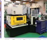
Wire Electric Discharge Machine (C-600iA)
