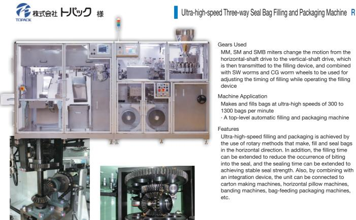
MM, SM and SMB miters change the motion from the horizontal-shaft drive to the vertical-shaft drive, which is then transmitted to the filling device, and combined with SW worms and CG worm wheels to be used for adjusting the timing of filling while operating the filling
