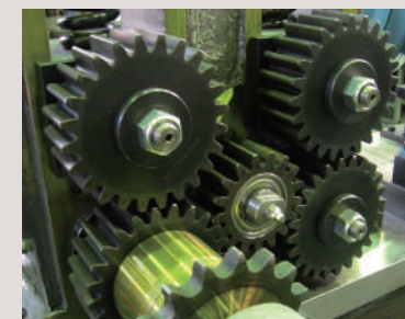
SS spur gears used for wire feeder
