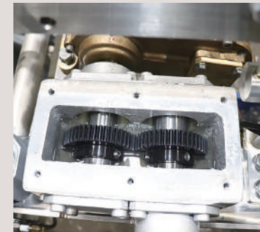
SS spur gears used for filleting fish
