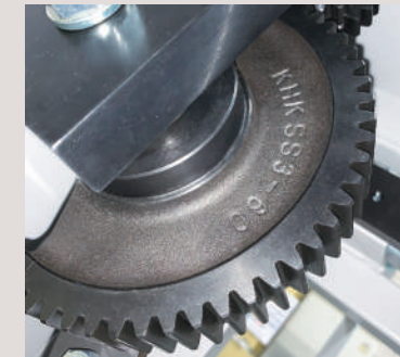
SS spur gears used in automatic carton formers
