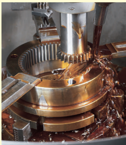
Gear cutting by CNC Gear Shaper
