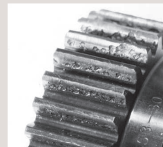
Example of wear due to insufficient surface durability
