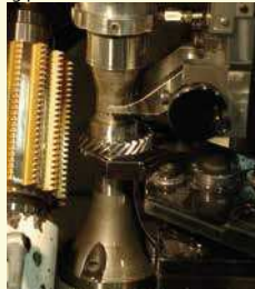
Gear cutting by a Hobbing Machine
